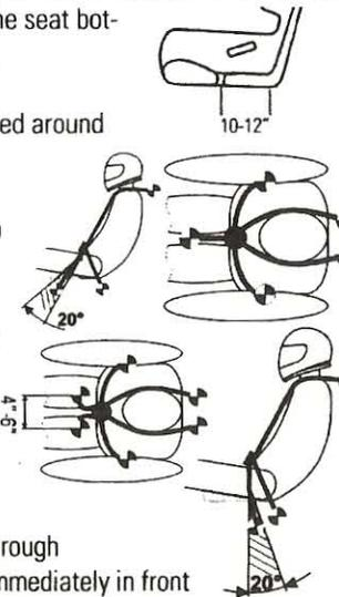
Note: FORMULA CARS where the driver is sitting on the sub-straps: Attach sub-straps rearwards in approximately the same location as the lap belts. This type of setup is typically used with a "Formula Style" or "Hybrid Style" looped sub-strap.
